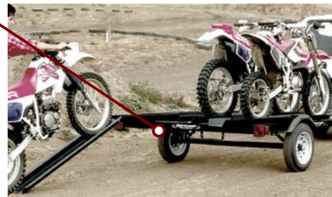
The removable ramp attaches quickly for easy loading. During travel, it stores neatly under the trailer frame and is secured with a locking pin.
