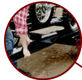
The removable ramp attaches quickly for easy loading. During travel, it stores neatly under the trailer frame and is secured with a locking pin.
